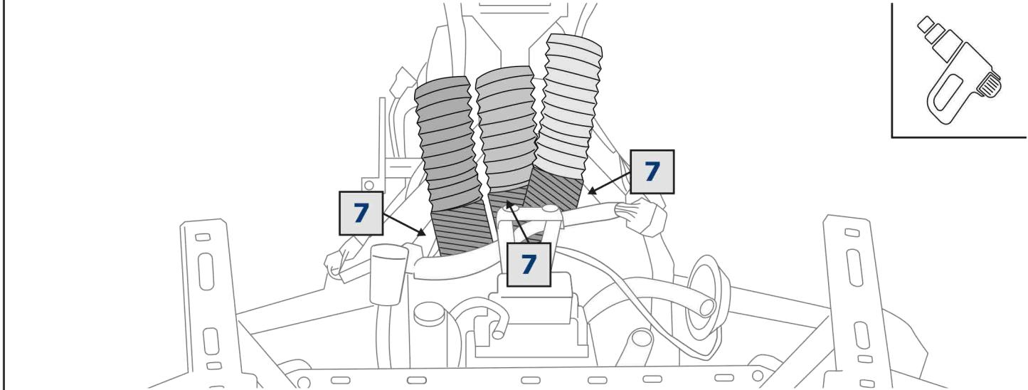
**EN** Install protective thermal hose ( $l = 0.1 \text{ m}$ ) on air ducts in such a way that the quad-bike steering column could not wear down them.
